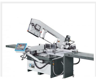
Powerful miter band saw for cuts from 60 ° right to 60 ° Left
