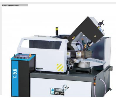
Electro-hydraulic automatic miter band saw for cuts from 0 ° to 60 ° left
