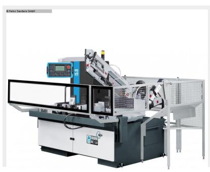
Powerful miter band saw for cuts from 45 ° right to 60 ° left
