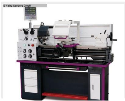
Fully equipped leading and tension spindle lathes. TH 3309D with digital position indicator DPA 21/3402040
